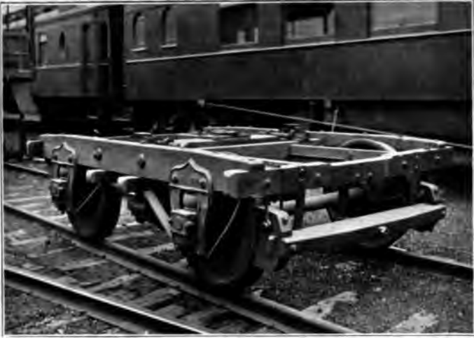
Type of wood-frame truck used on early cars; four wheels only, with a big rubber block over each in place of springs
